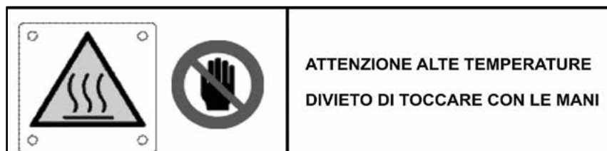
Fig. 2 - Security labels installed on the apparatus
